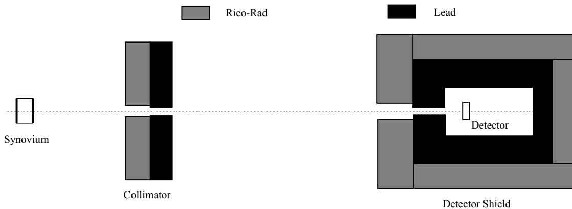
Figure 4.1 Schematic of the telescope system including photon detector, collimator for limiting the view angle of the detector to the synovium, and detector shield for reducing background counts and detector damage caused by fast neutrons.
