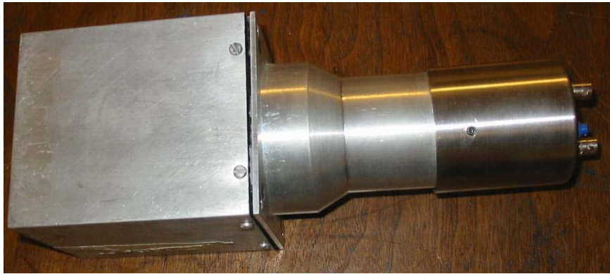
Figure 5.1 Picture of the NaI detector used in experiments. The 10.2 cm \times 10.2 cm NaI crystal and the PMT are encapsulated inside the aluminum shell.
