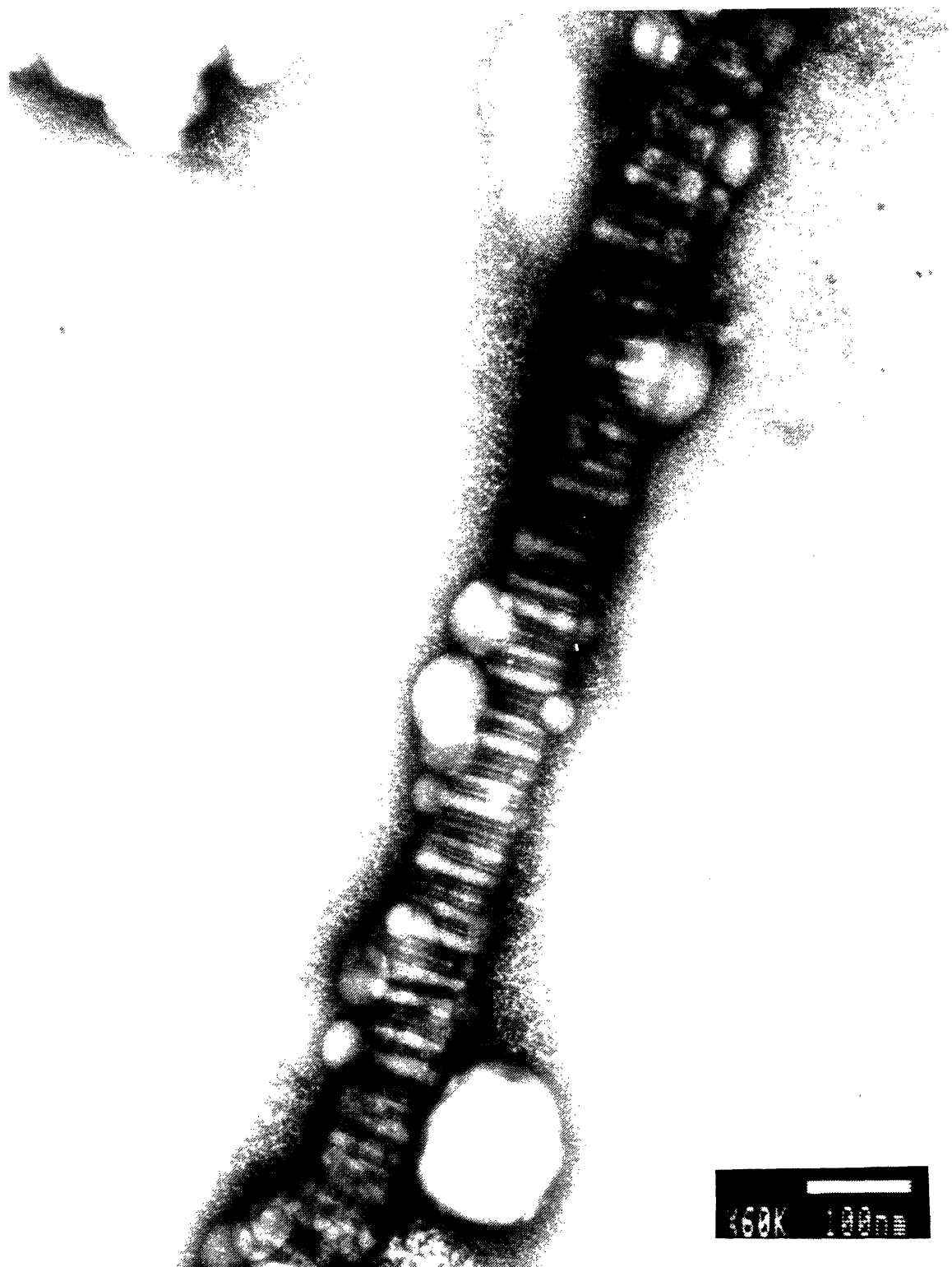
FIGURE 39 Electron microscopy of insoluble collagen suspended in phosphate buffered saline (60,000X magnification). Fibrils exhibit characteristic banded pattern; fibril diameter approximately 100 nm.
