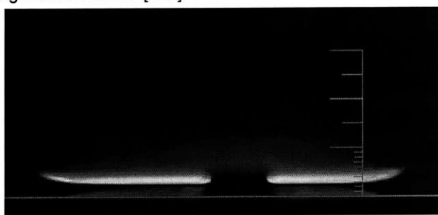
Figure 9.5. Major species and temperature profiles for a toluene-doped propane flame at \phi = 1.00 , pressure of 144 millibar, and unburned gas velocity of 20.3 cm/s. Flame image is shown at right; shadow in image is due to a bolt between the flame and camera.
