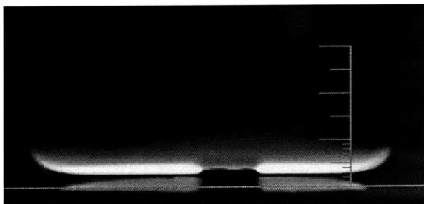
Figure 8.5 Temperature and species profiles from a propane-air flame at \phi = 1.20 . Filled symbols in the plots represent directly measured quantities; open symbols represent concentrations calculated via mass balance. The flame is shown in the image to the right. The horizontal line marks the burner surface at the flame center; each large scale division corresponds to 1 cm. Shadow at flame center is a bolt between flame and camera.
