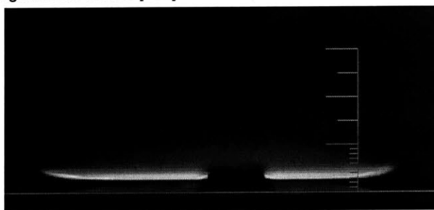
Figure 9.3. Major species and temperature profiles for a toluene-doped propane flame at \phi = 0.96 , pressure of 143 millibar, and unburned gas velocity of 20.5 cm/s. Flame image is shown at right; shadow in image is due to a bolt between the flame and camera.
