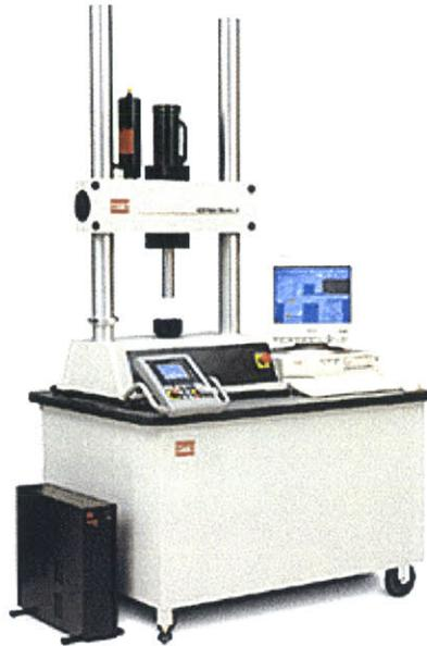
Figure 1-2. 858 Mini Bionix<sup>®</sup> II testing system (image taken from [9]).
