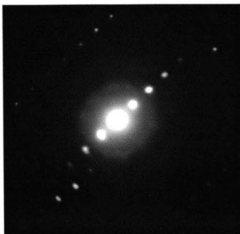
Figure 2-8: Selected-area electron diffraction pattern of the nanowire shown in Fig. 2-7.
