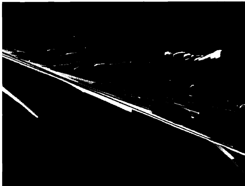
Figure 5. Polarized micrograph of the Col h phase of 3 (114.9 °C, 100x). The dark (pseudoisotropic) regions are areas where the columns are oriented perpendicular to the glass slide. The long needle-like regions are areas where the columns are laying more or less parallel to the slide surfaces.
