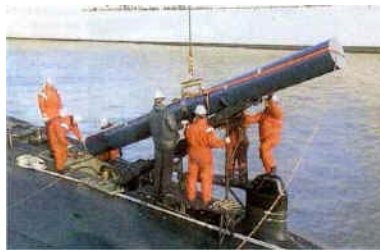
Figure 10. A Submarine Torpedo Room Berthing Pod being loaded into a Dutch submarine.
