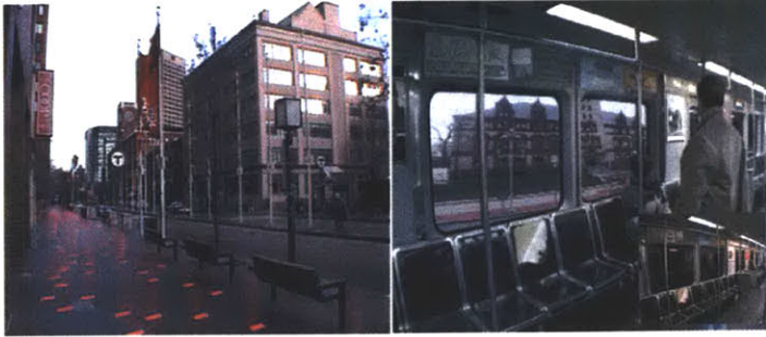
Fig. 4.10 Two renderings showing how an ambient information system could announce the arrival of the underground at Kendall Square in Cambridge, MA. Several bricks have been replaced by intelligent elements that would change color as the train arrives in the station underground. Meanwhile travelers in the train would be watching taped video feed of the landscape above ground to enhance their experience of the city. Reprinted with permission from Panagiotis Chatzitsakyris, Gonçalo Ducla-Soares, and Alejandro Zulas. "IN-Visible: Perceiving Invisible Urban Information through Ambient Media," CHI 2004 Vienna, Austria (24-29 April 2004).
