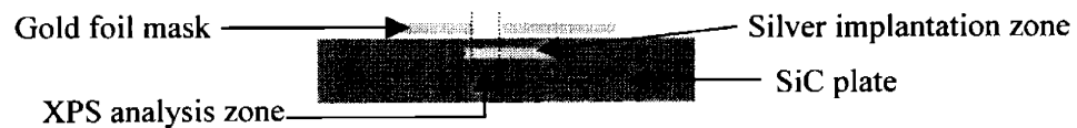
Figure 3-7. A gold-foil mask limited the XPS analysis area (schematic not to scale).
