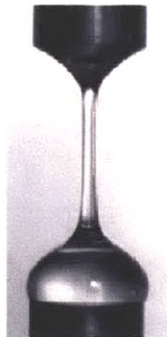
Figure 2-1: Liquid filament bridge is formed between two plates after application of a step strain.
