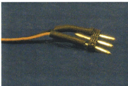
Figure 3.21: A simple humidity sensor.
