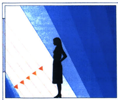
Figure 4.8: Note the area of darkness below the window in this schematic of light distribution.
