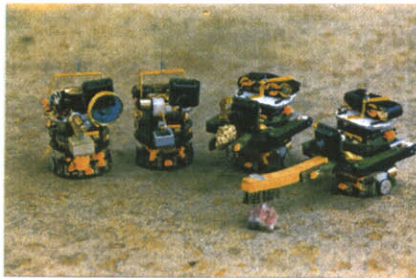
Figure 2.27: A group of Khepera robots used in several of Mataric's experiments, including those on forming flexible, adaptable robot formations.
