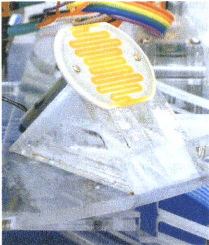
Figure 3.20: One of the photocells used as light sensors on the robots.
