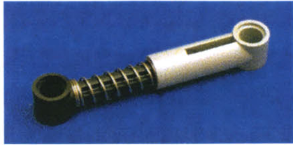
Figure 3.6: A LEGO suspension, modeled after traditional piston-and-spring styles.
