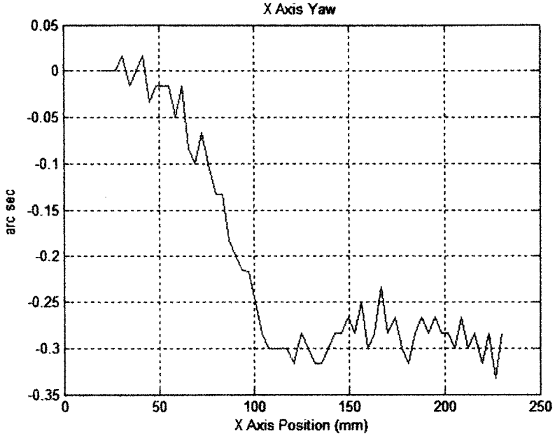
Figure 4-18 X axis yaw. 0.35 arc sec over 200 mm of travel.
