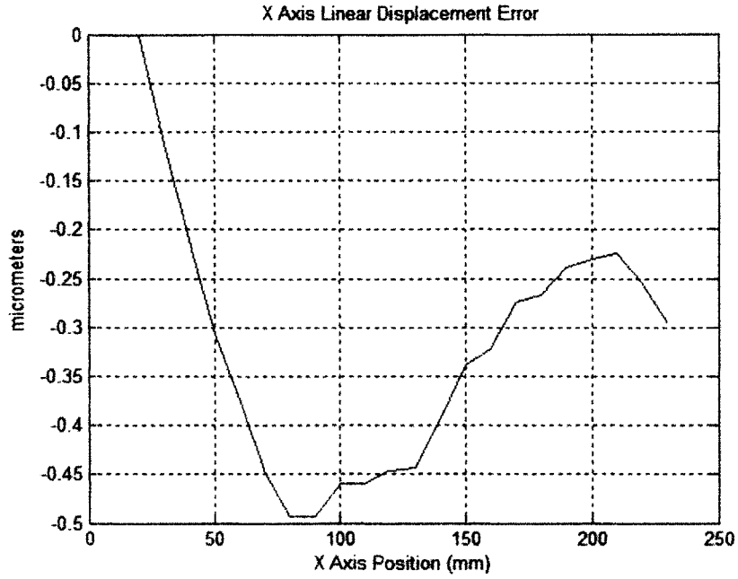
Figure 4-11 The X axis linear displacement error. The X axis is linear to 0.49 \mu\text{m} .
