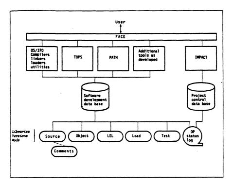
Software Factory Architecture. FACE = Factory Access and Control Executive; IMPACT = Integrated Management, Project Analysis, and Control Techniques; LEL = Link Editor Language; OP = Operational Program; PATH = Program Analysis and Test Host; TOPS = Top-Down System Developer. (Source: Bratman and Court, "Elements of the Software Factory," p. 129. Copyright © 1977 System Development Corporation [Unisys Corporation]. Reproduced with permission.)
