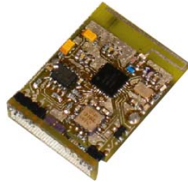
Figure 3-1 Transceiver with three axes of acceleration
