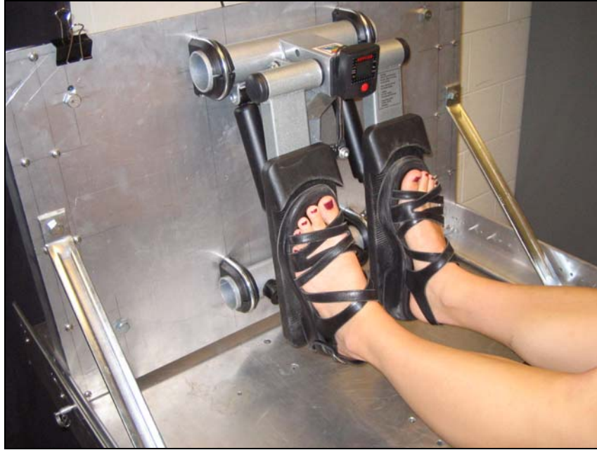
Figure 3.3. Close view of the new footplate, equipped with an exercising device.
