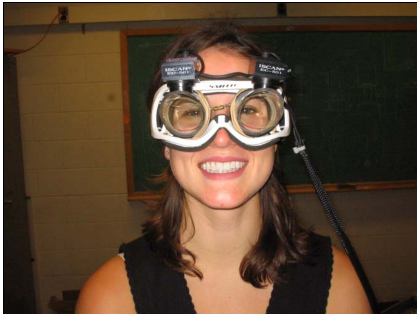
Figure 3.10. Happy subject wearing the new eye-movements measurement device, a ski-mask equipped with miniature cameras.
