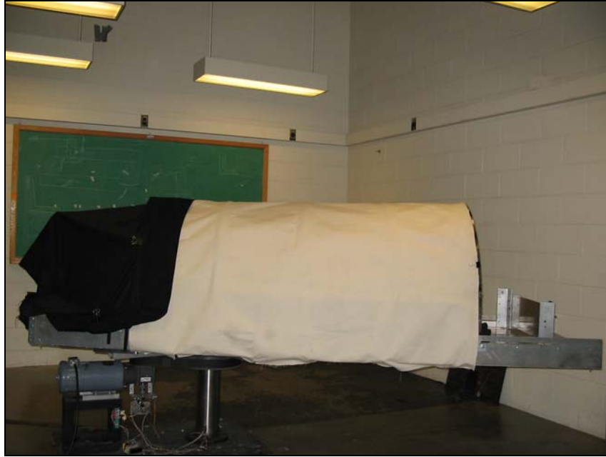
Figure 3.7. Archive view of the centrifuge equipped with the opaque canopy.
