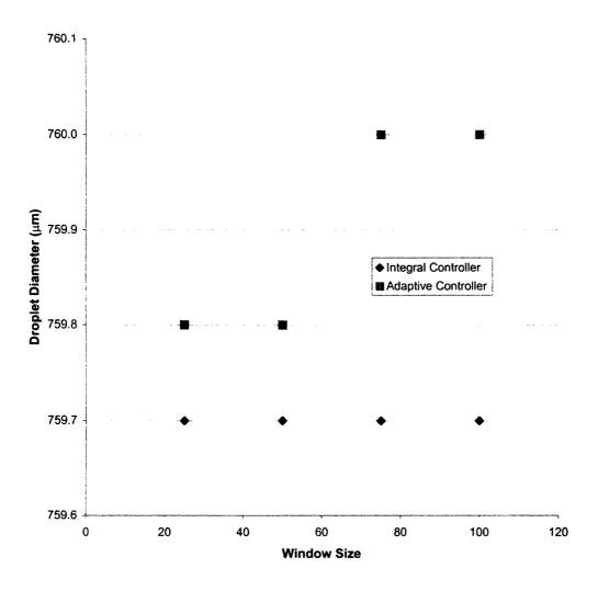
Figure 6: Effects of window sizing on the performance of integral and adaptive controllers. Target size is  $760 \mu m$ .
