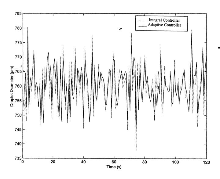
Figure 5: Comparison of an integral controller and an adaptive controller in the presence of Gaussian noise
