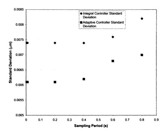
Figure 8: Effects of the sampling time on droplet diameter standard deviations
