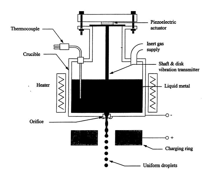
Figure 1: Schematic diagram of a uniform droplet generator
