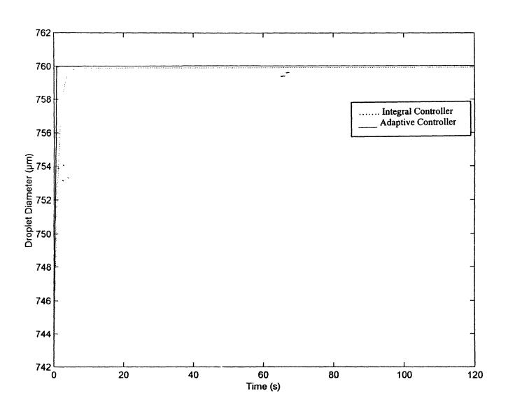
Figure 3: Comparison of an integral controller and an adaptive controller in the absence of noise
