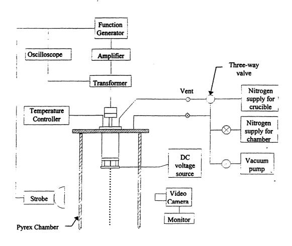
Figure 2: Schematic Diagram of a uniform droplet spray apparatus
