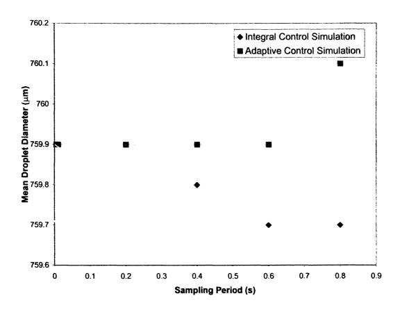
Figure 7: Effects of the sampling time on mean droplet diameters
