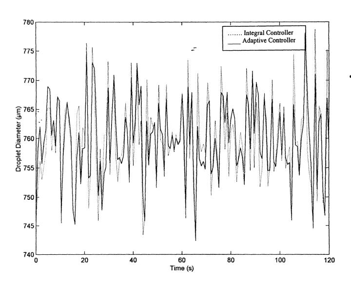
Figure 4: Comparison of an integral controller and an adaptive controller in the presence of white noise
