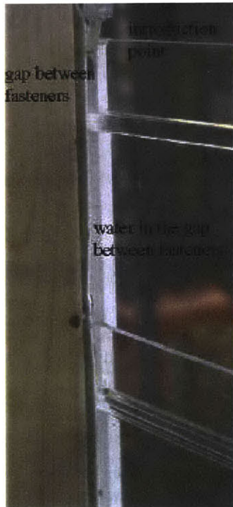
Figure 2-51 water in the gap between the fasteners
