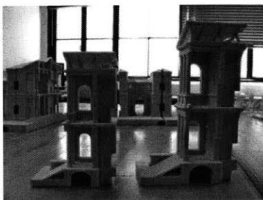
Fig. 33. 3D prints of Palladio building by Larry Sass presenting different scales derived from the same digital file.
