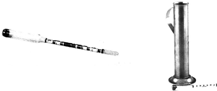
Figure 1: Matfer Salometer (left) and Matfer Syrup Density Meter (right, technically known as hydrometer)
