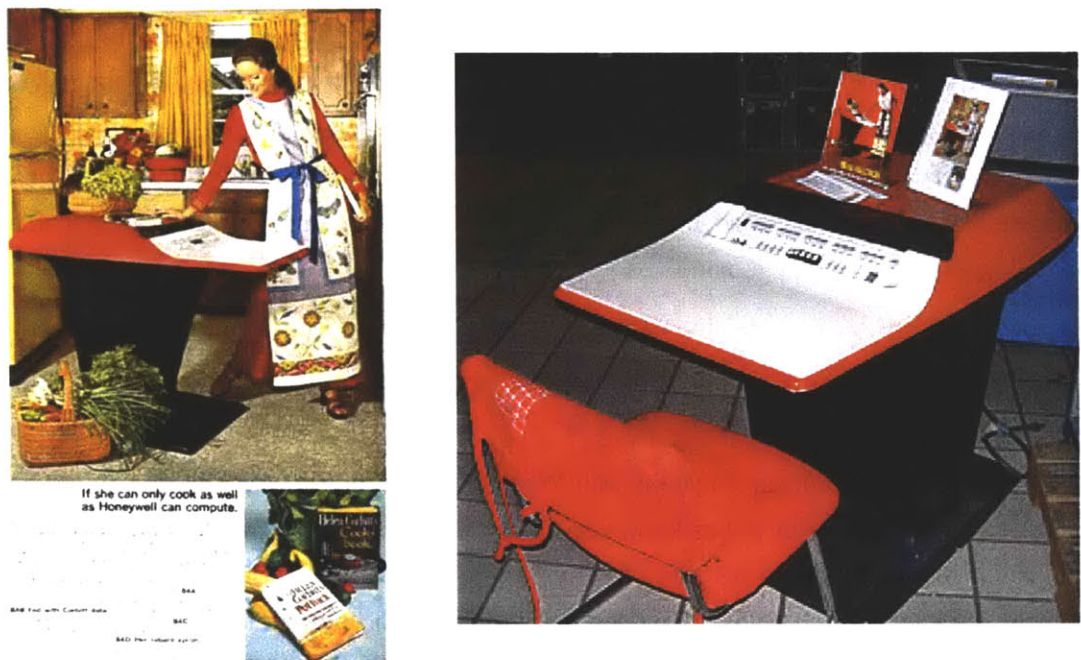
Figure 9: Honeywell H316 Kitchen Computer. The left shows a marketing brochure for the computer, "If she can only cook as good as Honeywell can compute." The right is a close up photo of pedestal version.
