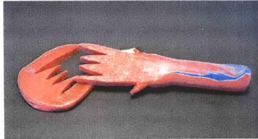
Figure 16: A model of the fork-spatula. The sensors will be embedded into fork, and the flap can be attached to the lower part of the fork and convert it into a spatula.
