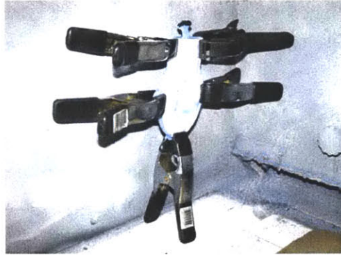
Figure 20: Filled mold in fume hood. The cramps hold the two pieces of the mold together while the silicone is curing.
