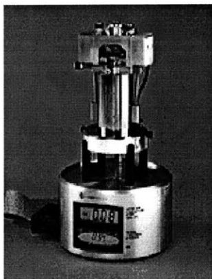
Figure 2-11: Veeco Multi-Mode Atomic Force Microscope, which was used in conjunction with a NanoScope® IV controller
