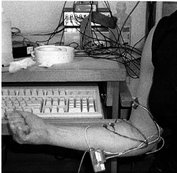
Figure 6-2. Subject 2 performs passive contraction test in the supinated forearm position, with the elbow held at 90° of static flexion.
