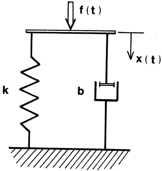
Fig. 1 — Damper — spring system
