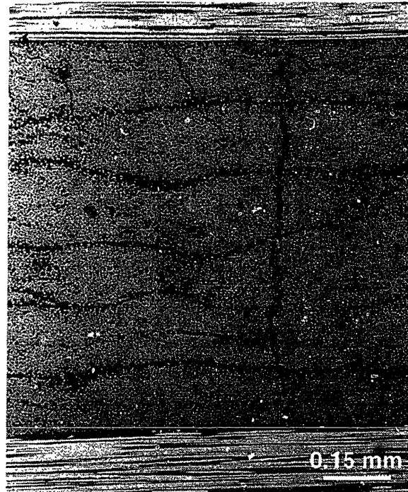
Figure 1.3: Edge damage in a cross-ply laminate exposed to 500 baseline cycles
