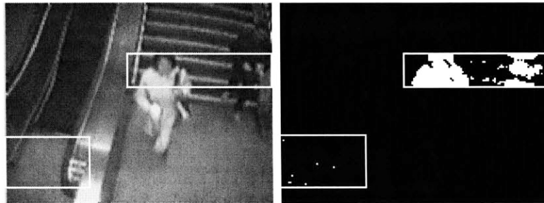
Figure 4-6: Real image and corresponding background subtraction image. Note that background subtraction is only performed in areas of interest that are highlighted.
