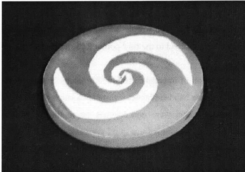
Figure 27. Fabricated Equiangular Spiral Slot Patch Antenna. 2.5 cm radius, 0.5 cm thickness.
