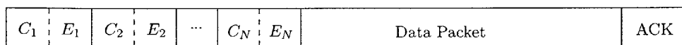
Figure 2-1: The signaling slots of the DCR protocol. The nodes are pruned through N contention-echo slot (CES) pairings.
