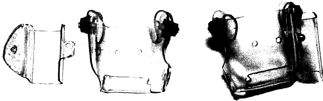
Figure D.27 GaitShoe attachment and battery enclosure; viewed separately from the back (left), and viewed together from the front (right)
