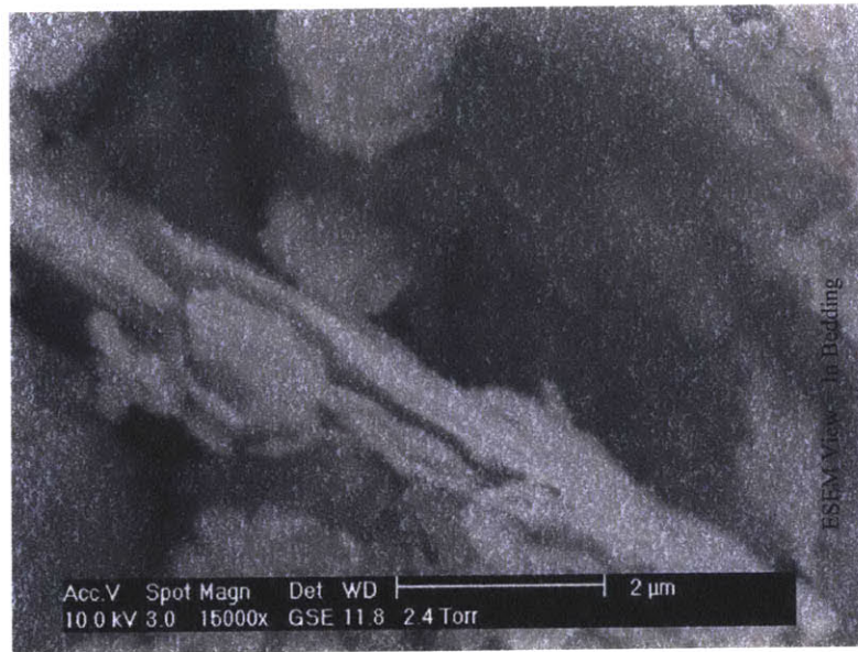
Figure 8-5: ESEM image Shale 1-2 (View in bedding direction): The image shows the elementary dimension of the mineral aggregates: length = 1000 nm; thickness = 100 - 250 nm.
