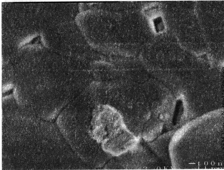
Figure 8-2: SEM-image of Shale 1-1 (View normal to bedding direction): The image shows the mineral aggregates of a characteristic dimension of 1000 nm.
