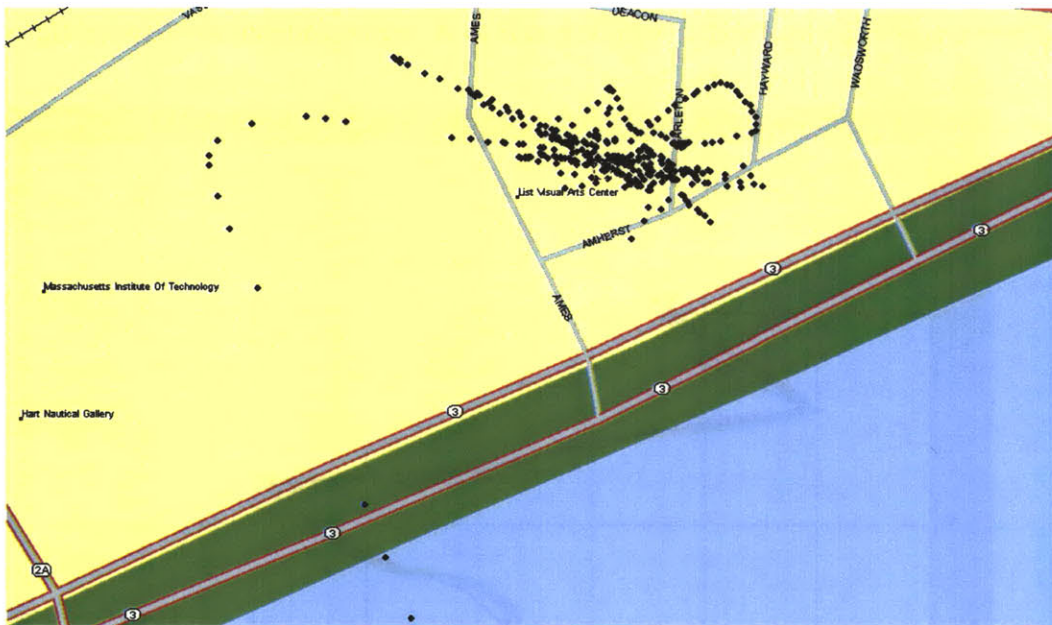
Fig. 4.4 Mapping of the GPS fixes recorded over the course of four hours from a static assisted GPS receiver.
