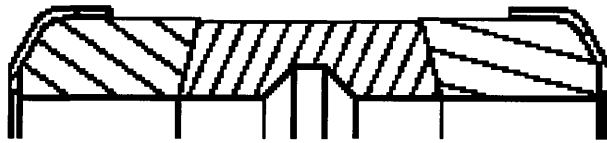
Figure 6. Cross-section of three-piece element with foldback ring
