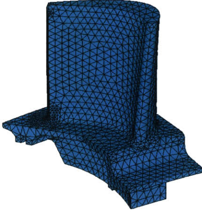
Figure 21 - Structural model solid elements - general view
