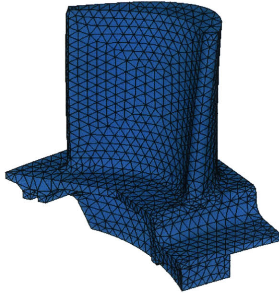
Figure 15 - Blade thermal model solid elements
