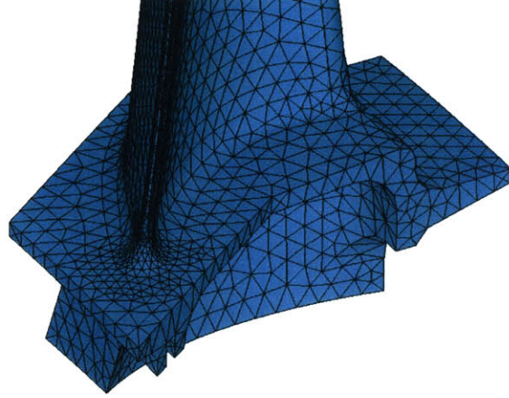
Figure 22 - Structural model solid elements - refined area in region of high stress and strain
