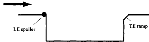
Figure 2-5: Various passive devices used for cavity tone suppression in literature and device location relative to the cavity.
