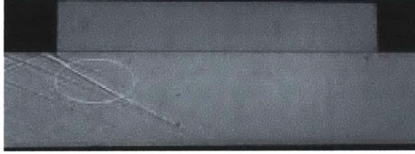
Figure C-2: Shadowgraph image for the FSU cavity corresponding to 30 psig microjet pressure. The encircled region was used for calculating the shock angle. External flow conditions: M = 2.0 and Re = 3 million (based on cavity length). Cavity dimension: L/D = 5.1 .
