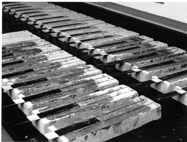
Figure 5.9 Fracture Specimens under Ambient Cure
