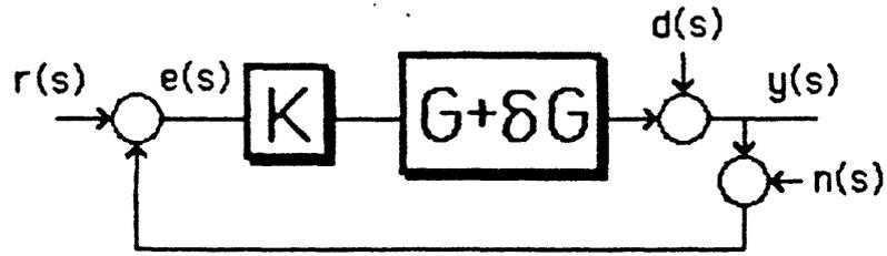
Figure 1: Generic MIMO Feedback Loop
