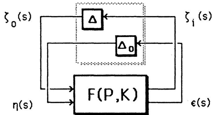
**Figure 5: Equivalence of Robust Performance and Robust Stability with Structured Perturbations**
