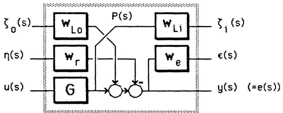
Figure 3: Internal Structure of P(s)
