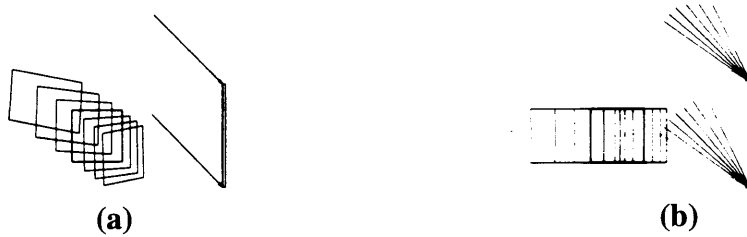
Figure 3.12: (a) Distortions of a square image across the visible spectrum (400-700 nm) (b) Single view angle dispersion compensation for reducing lateral chromatic aberration (Bazargan 1986, fig. 7.20)
