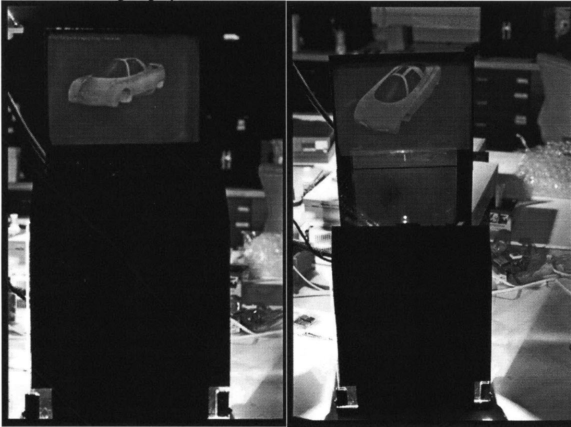
Figure 5.10: Plane-wave grating dispersion-compensation display (photos care of Michael Klug)
