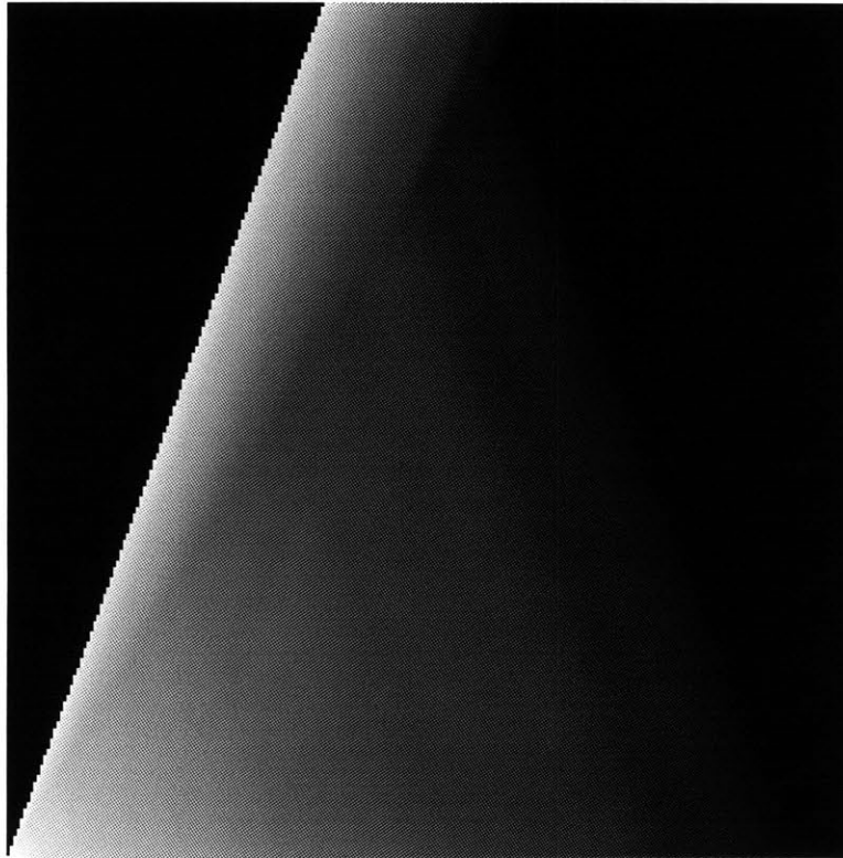
Figure 6-5: A quadrilateral decomposed into two triangles is prone to shading artifacts due to improper interpolation.
