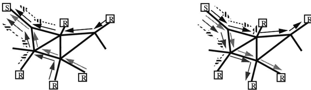
Figure 4-4 Effects of Late-Join Recovery on Server when using Unicast Transport
