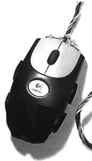
Figure 50: Pressuremouse, equipped with eight sensors: four foam sensors at the back of the mouse and two on each side.
