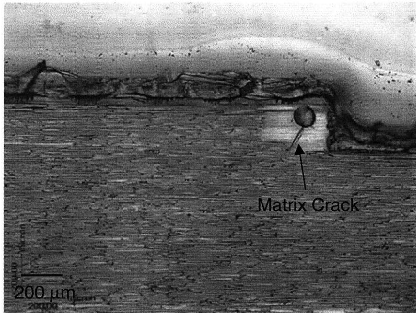
After Loading to 31.1 kN
