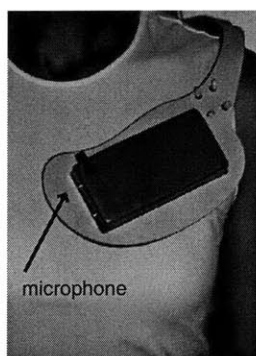
Figure 2-18: A “sociometer,” a portable audio/accelerometer/IR tag recorder developed by Tanzeem Choudhury, with the housing designed by Brian Clarkson. The microphone is about 6-7 inches away from the speaker’s mouth.
