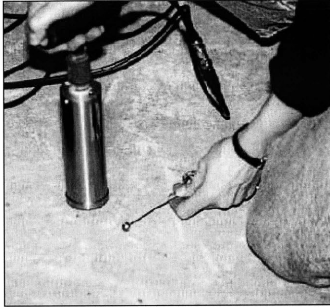
Figure 3. Inspector performing Impact-Echo test. Source: Carino 2001.
