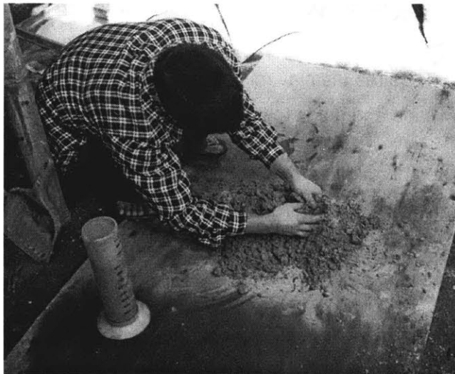
Figure 4.5: Worker Preparing a Mixture of Clay, Grog, and Water
