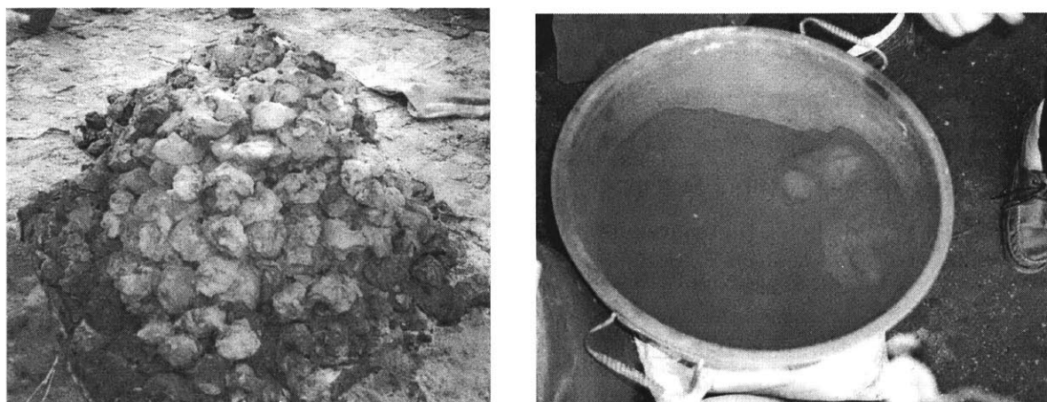
Figure 4.1: Raw Clay (left) and Processed Clay in Powder Form (right) used in the Production of Ceramic Water Filters at Madhyapur Clay Crafts
