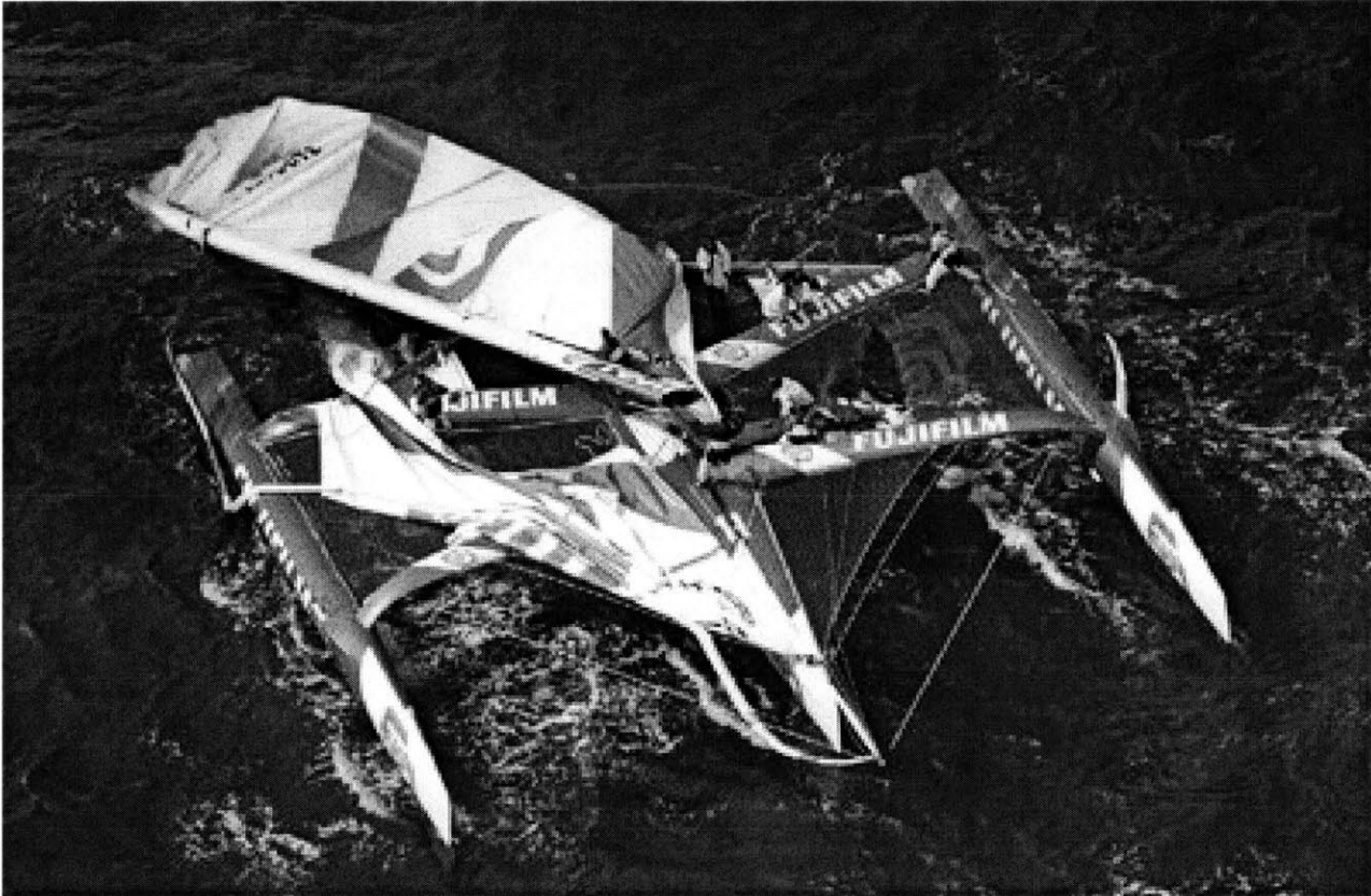
Figure 4.2 Trimaran “Fujicolor” after the break of its mast [28]
