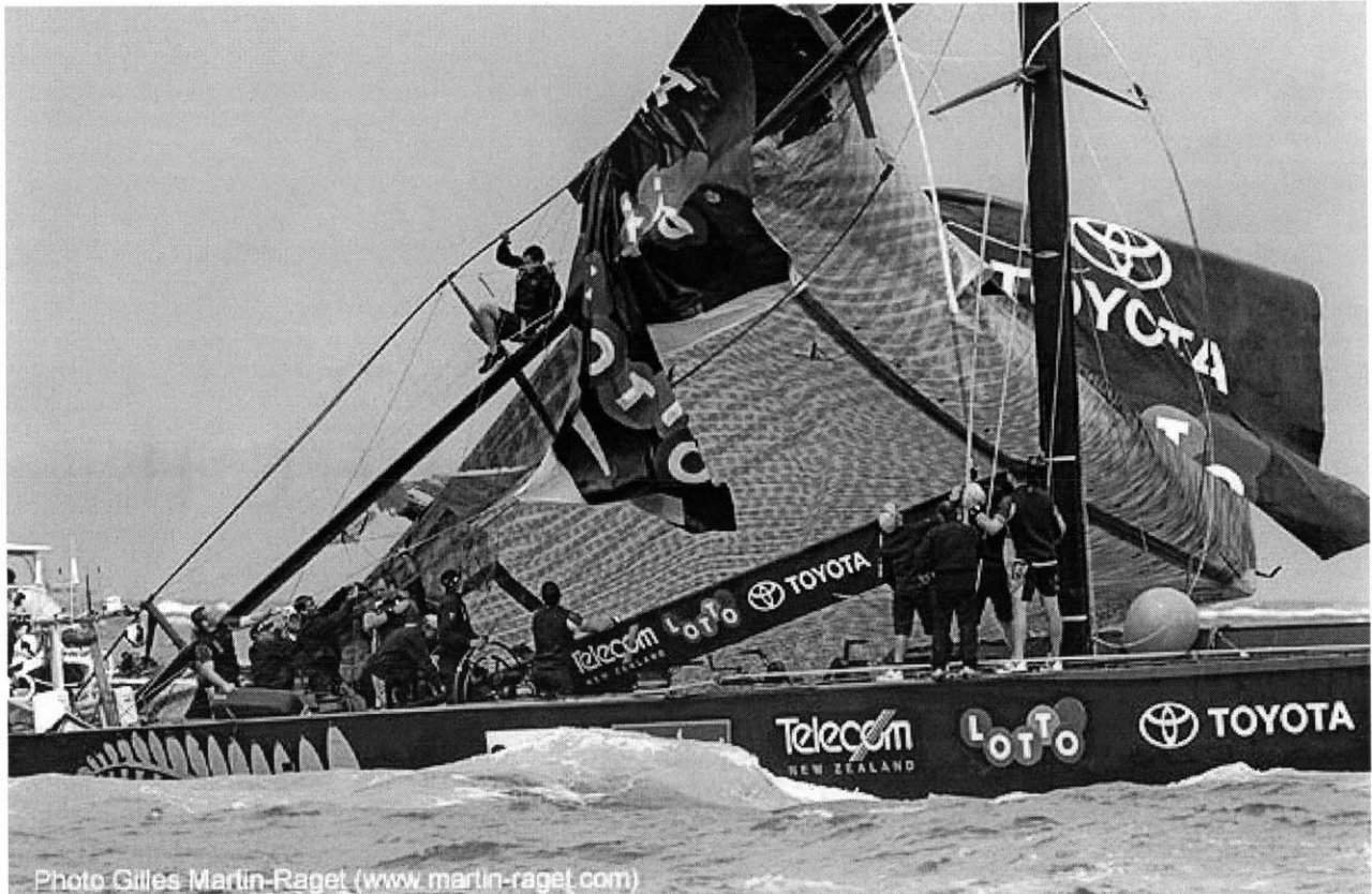
Figure 4.3 America's Cup finalist mast failure in 2003
