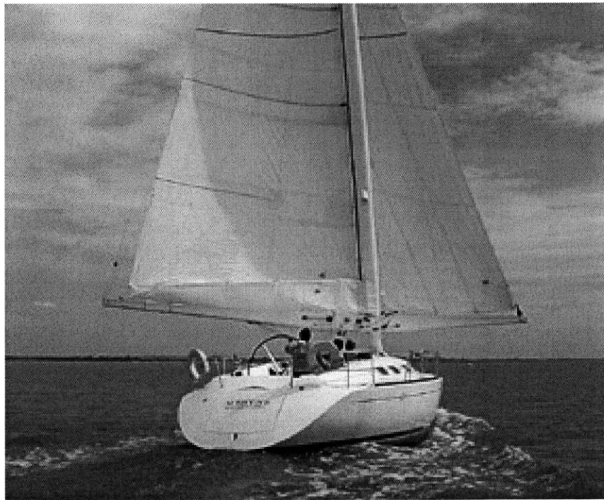
Figure 5.11 Beneteau 42s7 sailing yacht with free-standing mast [32]
