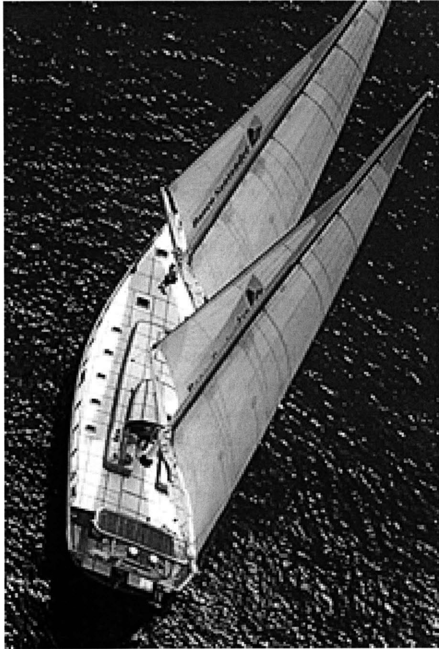
Figure 5.13 Cat-ketch yacht Paratii 2 with two free-standing masts [32]
