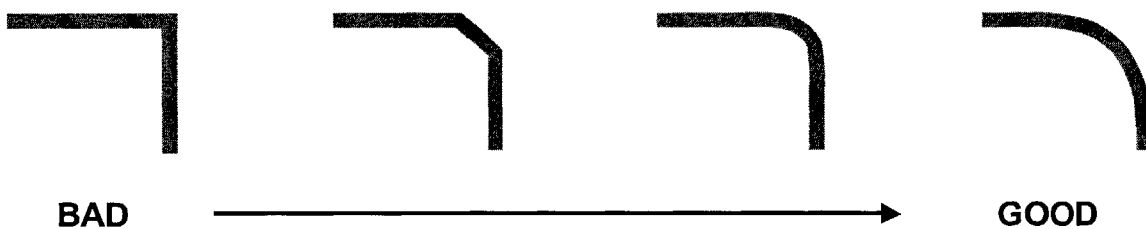
Figure 34 - A comparison of bends in transmission lines
