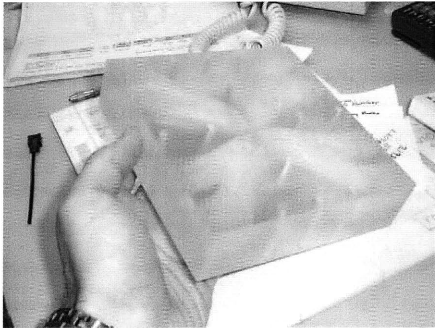
Figure 22 - A SLA block created with 512 tunnels
