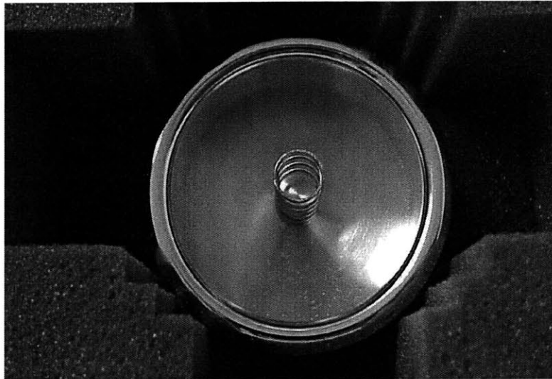
Figure 4.15 Diamond turned Nanogate load cap with spring.
