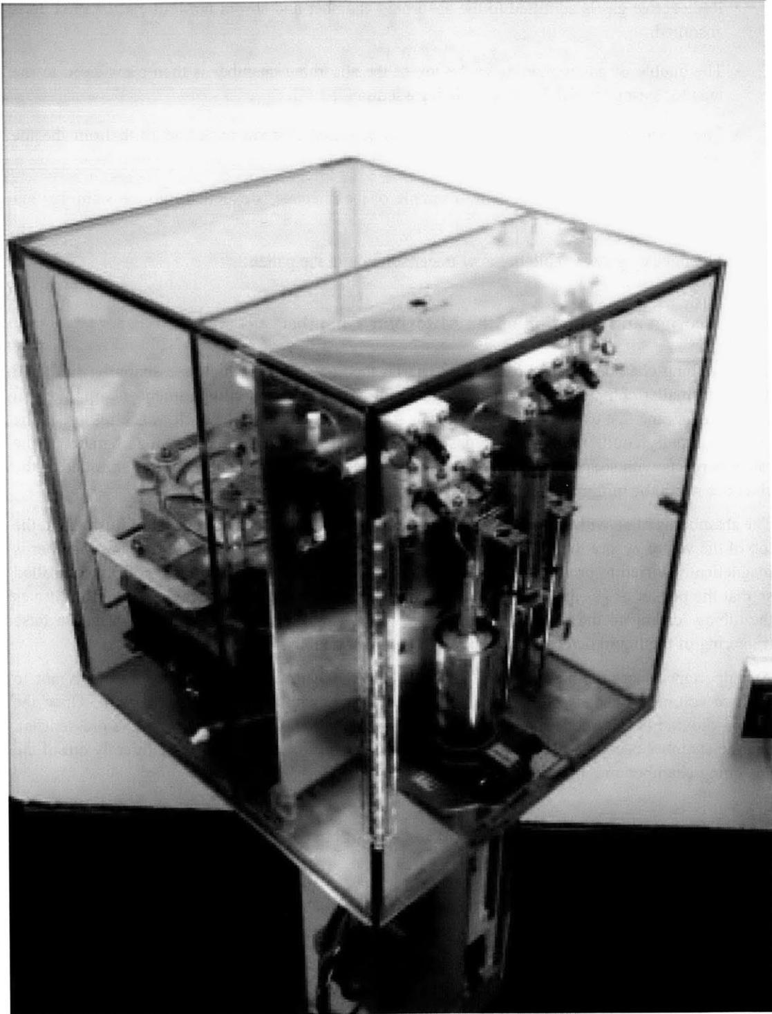
Figure 2.8: Oblique view of main unit. Enclosure is divided into three compartments. The front compartment contains the sterile components which are replaced for each subject. The central compartment houses the electronics. The rear compartment contains the absorbing chamber, dump tank, and other flow components .
