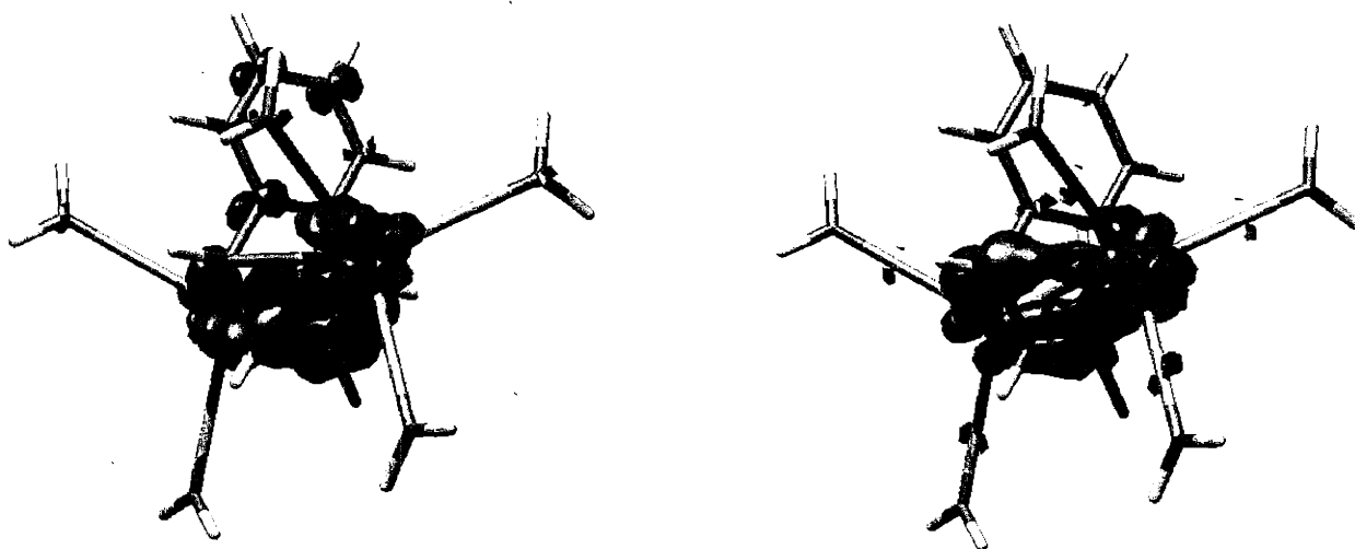
Figure 8. The two \delta -bonds ( \alpha component, \beta component not shown) between the uranium centers and the naphthalene fragment: SOMO-4 (left) and SOMO-5 (right).
