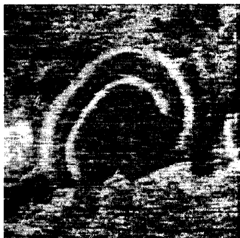
Figure 3-5: Sequence of 2 \times 2 \mu m in-phase SCA images taken in the central region of Figure 3-4. The scan at 3.98 Tesla has been signal averaged for a longer time than the others, and its signal-to-noise ratio is thus higher.
