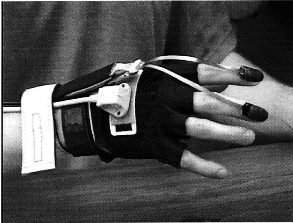
Figure 20: Finger-Free Electronic Glove with Fingernail Sensors Multiple fingernail sensors can be combined with other sensors such as the magnetic tracker shown here to form a fingerless glove.
