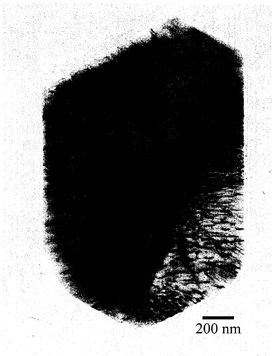
Figure 2.4 TEM Image of a typical \text{LiMg}_{0.05}\text{Co}_{0.95}\text{O}_2 particle used to prepare the suspensions at 34K magnification.
